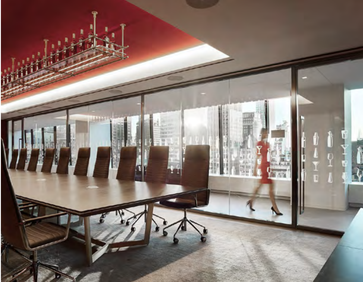
NEW YORK HEADQUARTERS OF A LEADING MULTINATIONAL BEVERAGE COMPANY; 2000 METERS OF DEMOUNTABLE GLAZED PARTITION WITH CUSTOM SCREEN-PRINTED GLASS;
